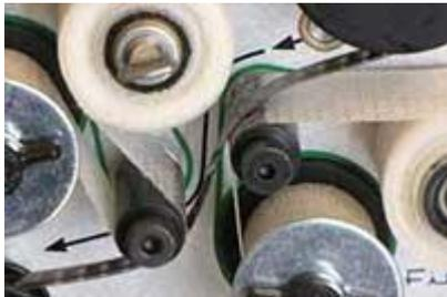
method, takes place just before the film frame is capture. The film is taken through cleaning rolls wet with "Filmrenew". This cleaning process traps dust and unwanted dirt particles. Most transferring houses offer the cleaning as an option with extra charge.
